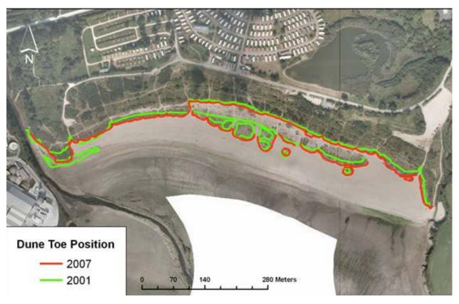
Figure 3.4 Dune toe positon at Par Sands in 2001 and 2007 (source: Halcrow, 2009c).
