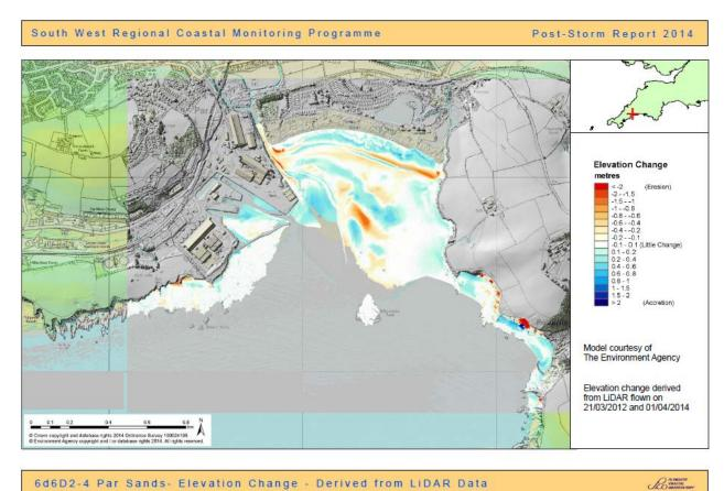
Figure 3.10 Post storm elevation change at Par Sands (source: PCO, 2014c).
