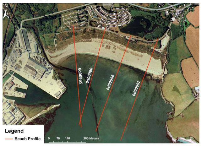
Figure 3.5 Diagram showing position of SWRCMP beach profiles at Par Sands.
